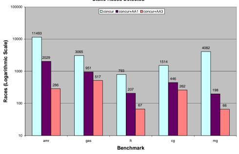
Fig. 8. Number of data races reported for different levels of analysis.
